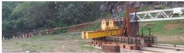
Test Rig for Qualification Tests on ERS Panels
