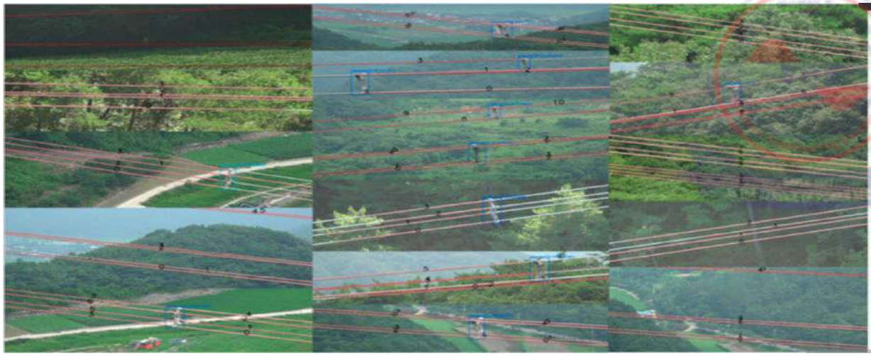
Figure 5. Power line detection results. The proposed power line detection algorithm shows robustness against cluttered background and different lighting conditions. Detected power lines are marked in red and labelled with ID numbers.
