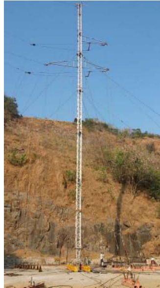
ERS Test Set-up Deformed Shape of ERS
