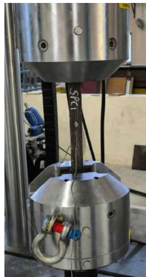
Tension Coupon Test (ASTM E8) – Test Setup
