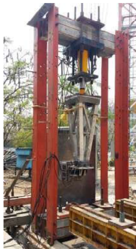
b) Transverse/Shear Test Tests on Gimble Joint and Bottom Panel
