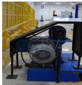
Torsional Ductility Test Setup
