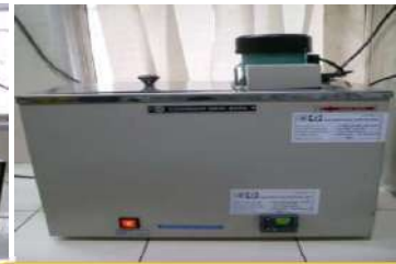
Constant Temperature Bath for Oil separation test on grease.
