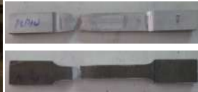
Coupon Specimen Failure Pattern
