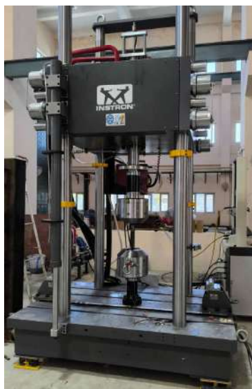
Tension Coupon Test (ASTM E8) – Test Setup
