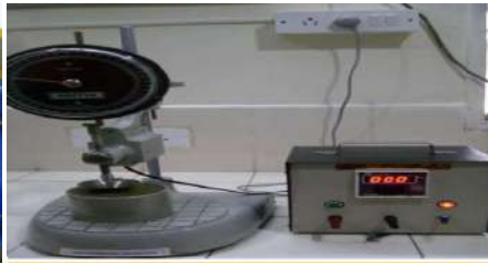
Core Penetrometer for grease.
